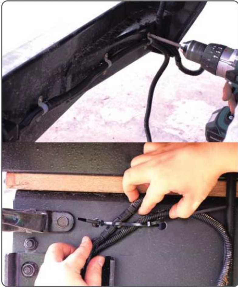
17. Organize Transmitter/Rear camera cables.
