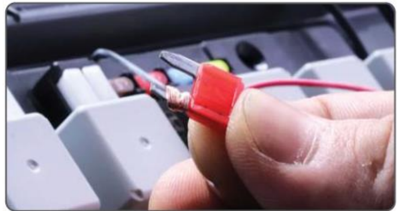
24. Detach the fuse and wrap power wires.
