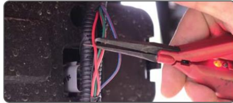
14. Strip rear lamp & ground wires.
