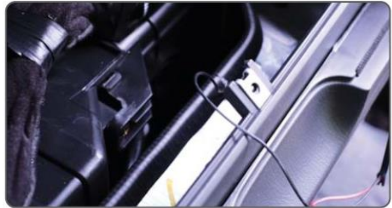
22. Attach the receiver ground cable to the surface.
