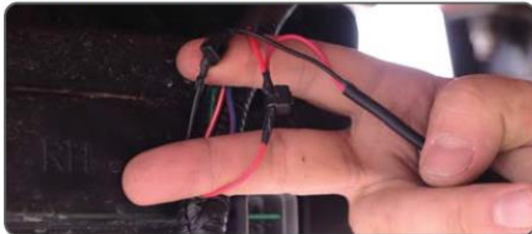
15. Connect transmitter cables to the rear lamp & ground wires respectively.
