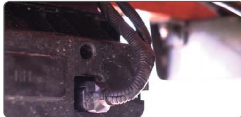
16. Attach the rear lamp connector.
