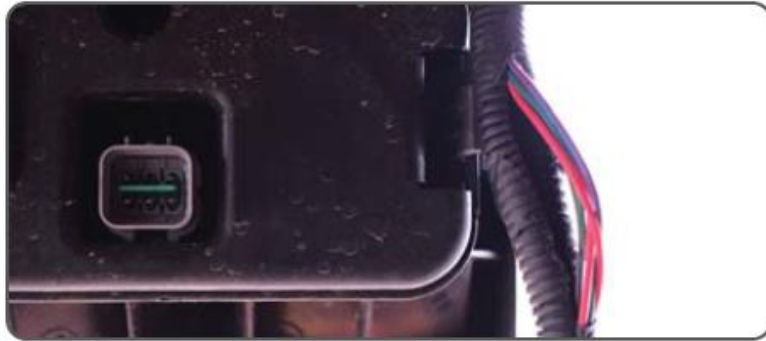
13. Detach a rear lamp connector.
