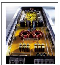
High quality electronic in-ternal design with double-sided FR4 epoxy circuit boards and premium components.
